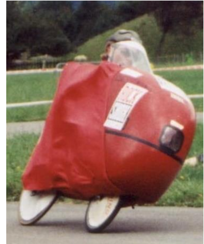
Figure 6: Lightning F-40 with fairing
